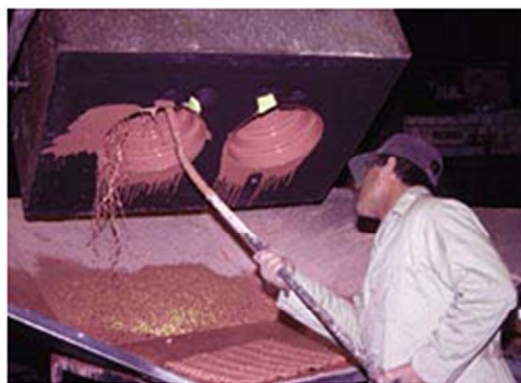
Figure 6. Flow coating method, it is seen that the mould is inclined at an angle.
