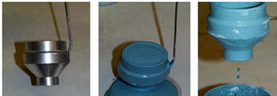
Figure 8. Measurement of viscosity with a flow cup [45].
